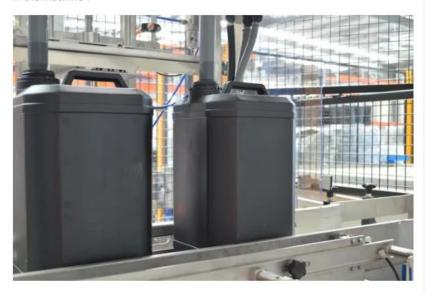
The machine fills by weight, instead of by volume, which further helps with consistency and reduces wastage.
